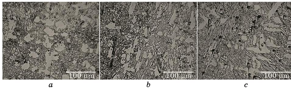
Fig. 7. Effect of Ti content on microstructure of chromium–manganese cast iron: no Ti (a), 0.49% Ti (b), 0.87% Ti (c).
