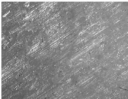
Fig. 1. Friction surface of steel 45 in dynamic mode when moving on glass without the influence of a magnetic field.
