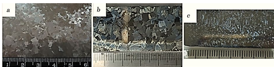
Fig. 2. Macrostructure of alloys after etching: a —alloy No. 1, b —alloy No. 2, c —alloy No. 3.
