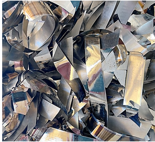
Fig. 1. Non-conforming remnants of the studied amorphous alloy MM-11H ribbon.
