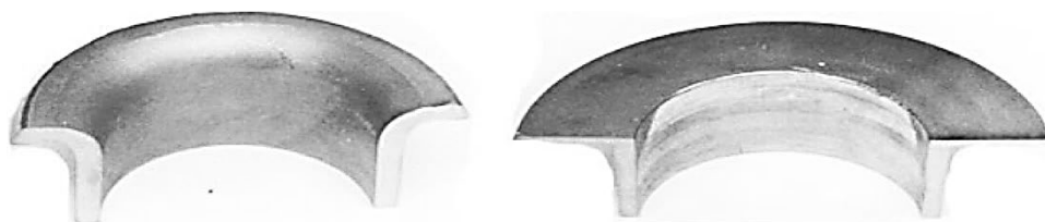
Fig. 7. The workpiece obtained by debarring: at the intermediate and final stages.
