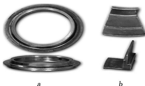
Fig. 9. Complicated profiled products obtained by rolling with a cylindrical roll: a —flange with a collar; b —element of the body of the electrovacuum device.
