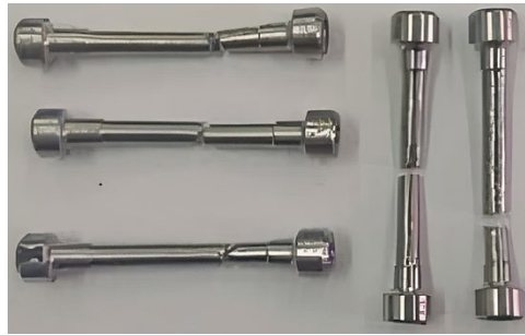
Fig. 7. Broken samples after tensile testing at room temperature.
