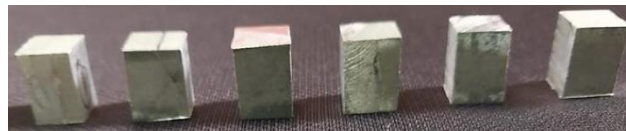
Fig. 4. Pin samples for tribological testing.
