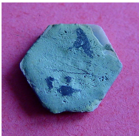
Fig. 3. \text{ZrO}_2 -ceramics metallised with \text{Al}_3\text{Ti} after annealing in air at 1000^\circ\text{C} during 60 min.
