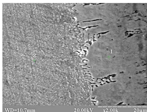
Fig. 3. Electron microscopy of 38Cr2MoAl steel after complex chemical-thermal treatment according to mode No. 2, which consisted of carburization followed by boriding at temperature of 850°C for 2 hours (Table 1).
