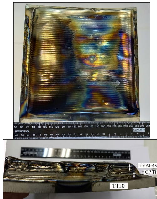
Fig. 1. Top and side view of manufactured 3-layer plate.
