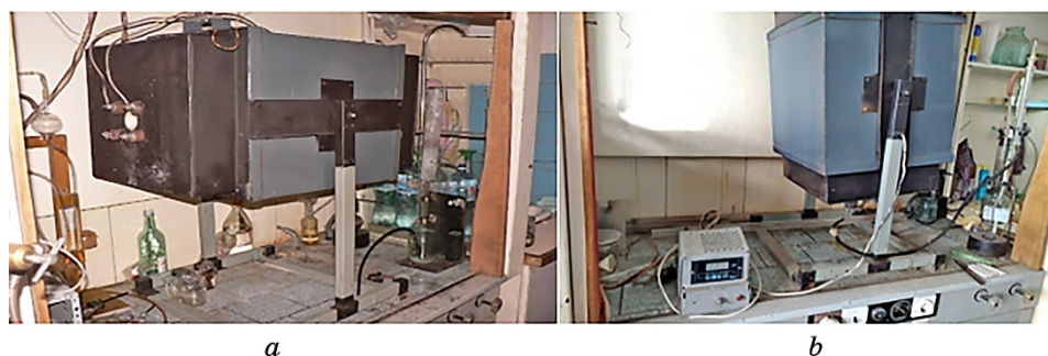
Fig. 2. Pyrolytic equipment with a reactor: in a horizontal position ( a ), in a vertical position ( b ), schematic representation of the equipment for the pyrolytic synthesis of CNS when using a horizontal type reactor (1—thermal insulation of the pyrolysis furnace, 2—furnace heaters, 3—reactor inlet flange with thermocouple, 4—directed flow of hydrocarbon gases, 5—axis of the reactor, 6—quartz reactor, 7—catalyst layer, 8—pad, 9—synthesized CNSs, 10—directed flow of gases for utilization, 11—outlet flange of the reactor) ( c ), the principle of operation of the equipment for CNS pyrolytic synthesis when using a vertical type reactor (1—directed flow of hydrocarbon gases, 2—nozzles for supplying solutions, 3—the direction of gravity flows, 4—furnace heaters, 5—thermal insulation of the pyrolysis furnace, 6—quartz reactor, 7—axis of the reactor, 8—carbon nanostructures, 9—platform for collection CNS, 10—reactor flange, 11—supply of hydrocarbon gases, 12—synthesized CNS) ( d ).
